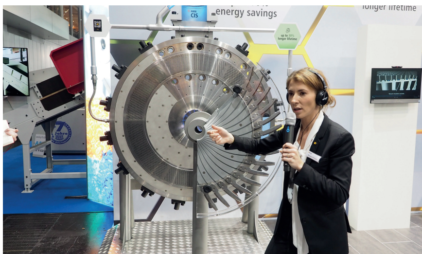
Fig. 2. The AMN cutting head system with central water injection from Maag ensures permanently high pellet quality. © Hanser/Schröder
